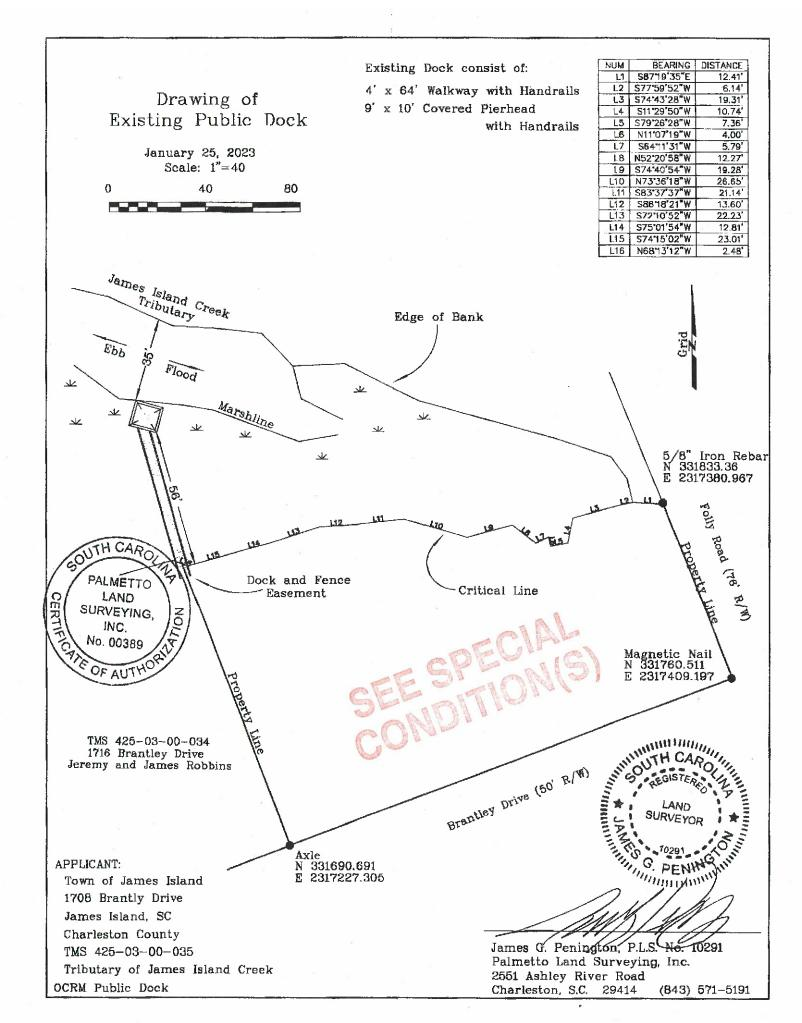
Patterson Ave Existing Dock consist of: 4' x 64' Walkway with Handrails 9' x 10' Covered Pierhead with Handrails SITE Proposed Work consists of: Brantley Drive Reconstructing 4' x 64' Walkway with Handrails Reconstructing 9' x 10' Covered Picrhead Santee Street with Handrails Vicinity Map NTS -- 104' critical 72' 9' x 10' Covered Pierhead 4'x 56' Walkway 3' min. marsh MHW **PALMETTO** LAND Drawing of SURVEYING, Public Dock Reconstruction INC. No. 00389 January 23, 2023 Not To Scale To Scale
