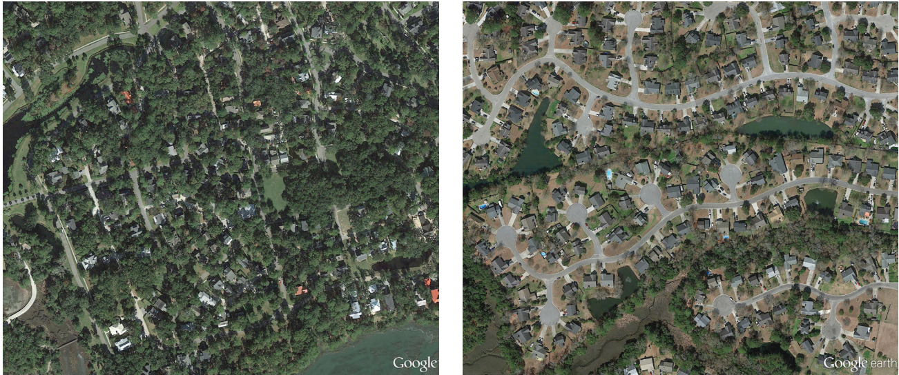
Figure 3.2-3. Aerial image comparison of two developments with quarter-acre lots: (A) is from Beaufort, SC (~25% impervious surface) and (B) from Mt. Pleasant, SC (45% impervious cover). Images from Anne Blair, NOAA Hollings Marine Laboratory, and Google Earth.
