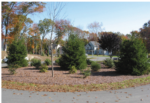
Figure 4.2-2. Bioretention in a Cul-de-sac (Photo: Center for Watershed Protection)
