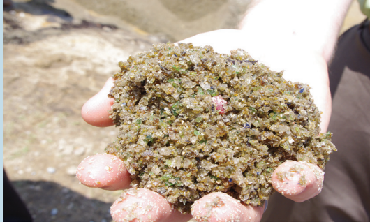
Figure 5.2-1. Soil media mixed with recycled glass product from the Horry County Solid Waste Authority. (Photo: Clemson Carolina Clear)
