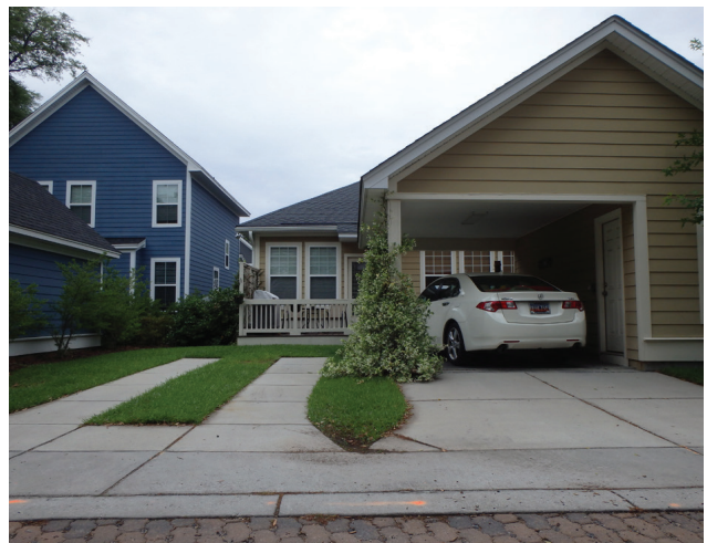
Figure 3.3-4. Oak Terrace Preserve in North Charleston required a maximum of 50% impervious cover on lots. In order to remain under this threshold, the independent contractors developed inventive driveway designs. (Photos: Lisa Vandiver, NOAA Restoration Center)
